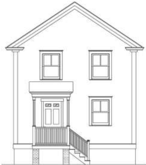
▲ Inappropriate Brick or wood columns without infill.
