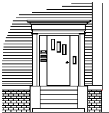
▲ Inappropriate Sidelights replaced by mailboxes and buzzers.
