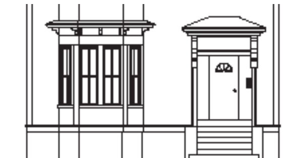
▲ Inappropriate Single door instead of double door. No panels. Non-historic glass panel design.
