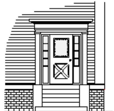
▲ Inappropriate Door design and aluminum screen.
