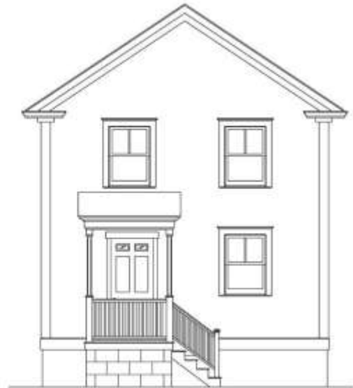
▲ Inappropriate Cinderblock porch base.
