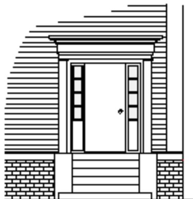
▲ Inappropriate Door without panels in wood, steel, etc.
